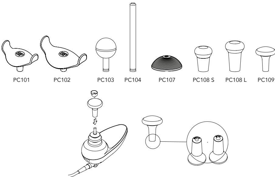
**en** All Bodypoint Joystick Handles with flexible shafts will, by design, slide off of the steel joystick stem if subjected to undue pulling. The U-shaped Joystick Handle design also allows rotation on its shaft. These design features are meant to prevent damage to the joystick box. Altering the product to circumvent these features is not recommended. Our Joystick Handle is designed with a flexible shaft that will fit tightly on any 3/16" (5 mm) or 1/4" (6mm) diameter steel joystick stem.
